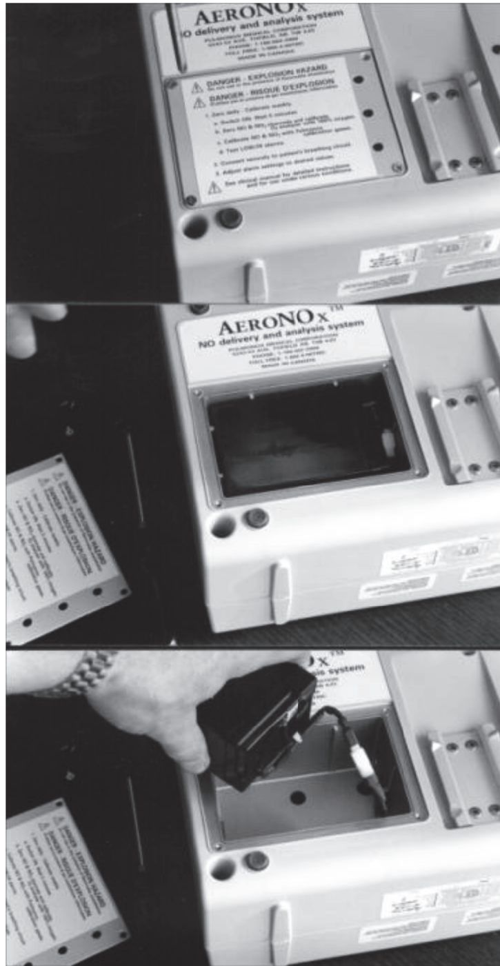
Figure 4-1 BATTERY REMOVAL / REPLACEMENT
