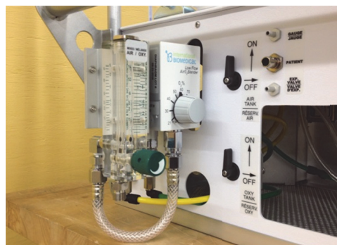
Figure 2 - 5 Blender / Flowmeter Hose Connection
