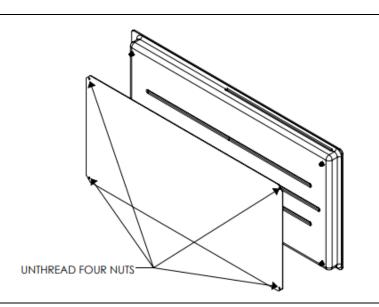
6. Separate the patient tray from the aluminum deflector panel by unthreading the 4 nuts at each corner of the tray.
