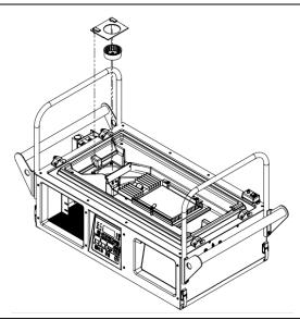
Remove the impeller guard by toggling the black swell latches (2) in the up position and then pull up on the impeller guard. Once exposed, pull the impeller off the motor shaft.
