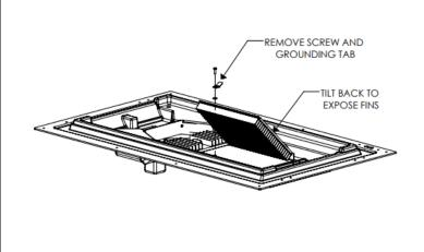
8. Using a Philips head screw driver, remove the front screw, washer and grounding tab securing the heat sink. Rotate the heat sink back to expose the fins for cleaning.
