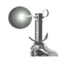
4)Apply magnifying glass if needed by rotating it to a proper position.
